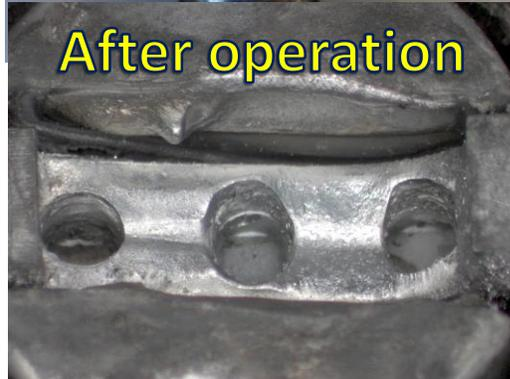
The discharge power of 2 – 4 kW (pulsed) is distributed across the 2 x 49 mm<sup>2</sup> surface area
