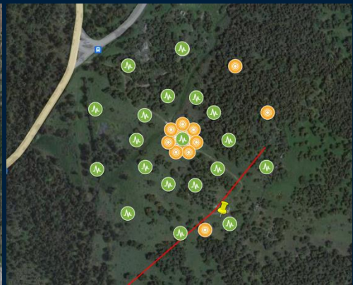
P2 broadband array + geophones (September 2021)
