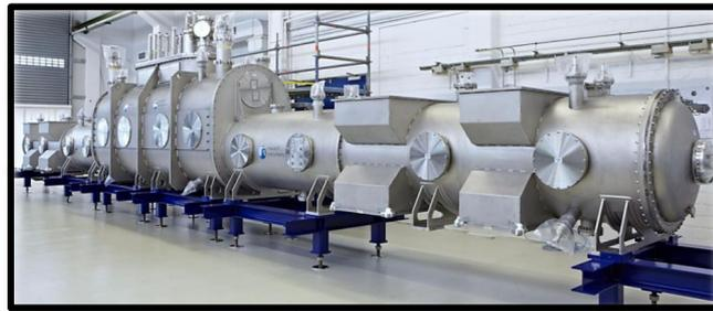
Windowless Gaseous Tritium Source cryostat
