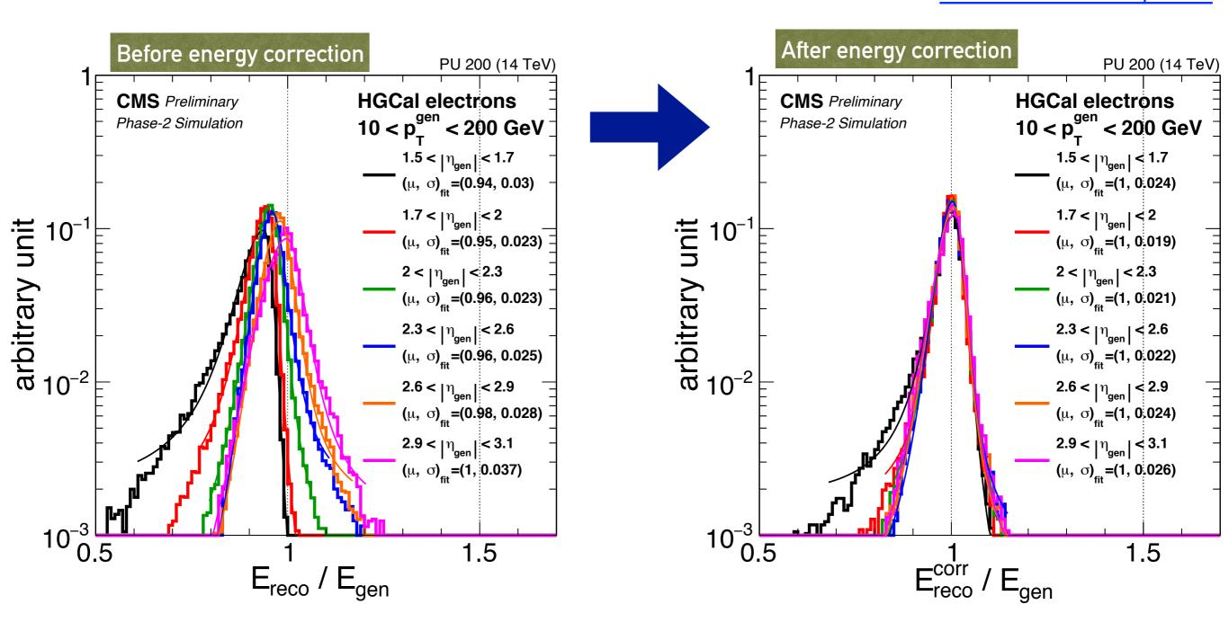
Satisfactory energy response and resolution after regression-based energy correction Response & resolution stable across the whole  $|\eta|$  range of HGCAL.
