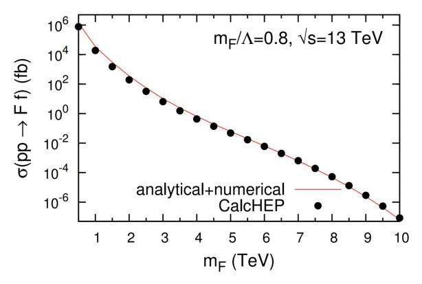
Good agreement between analytical+numerical calculation and the results of the CalcHEP simulation, which validates the model implementation
