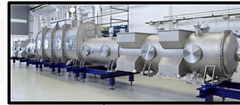
Windowless Gaseous Tritium Source cryostat
