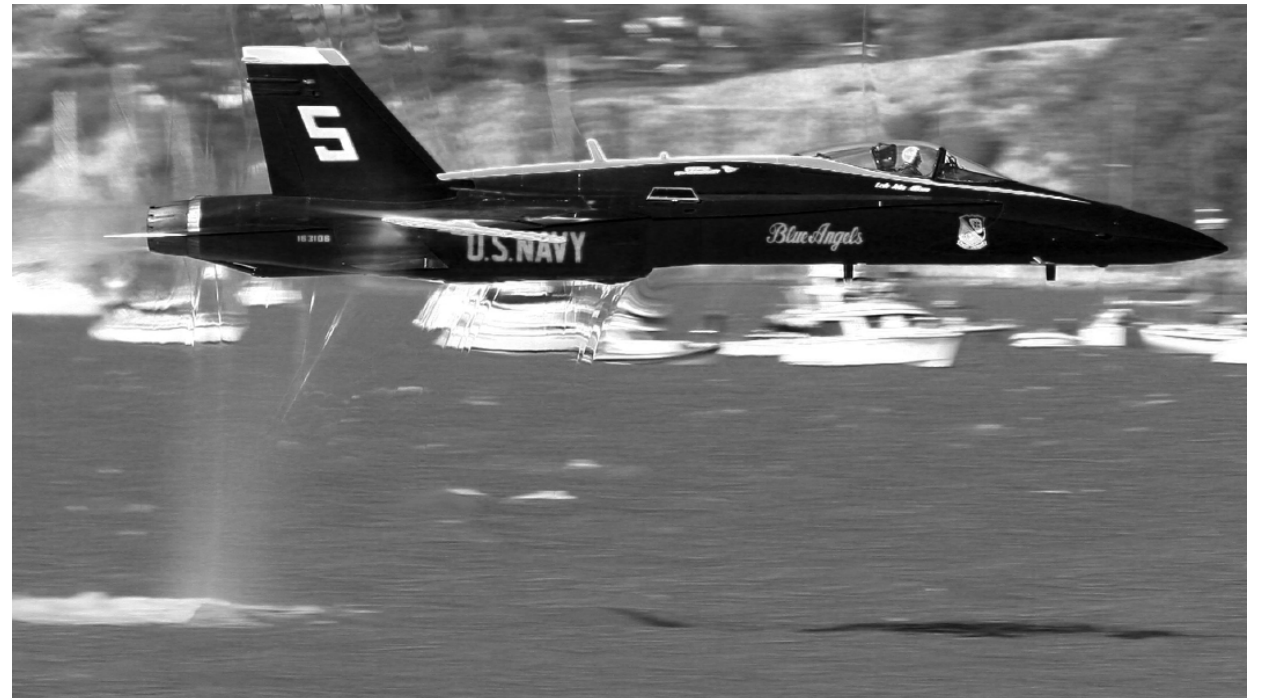
Figure 1. A US Navy Blue Angel demonstration aircraft during a Mach 0.95 pass, highlighting shock/surface interaction (with permission: Matt Niesen).
