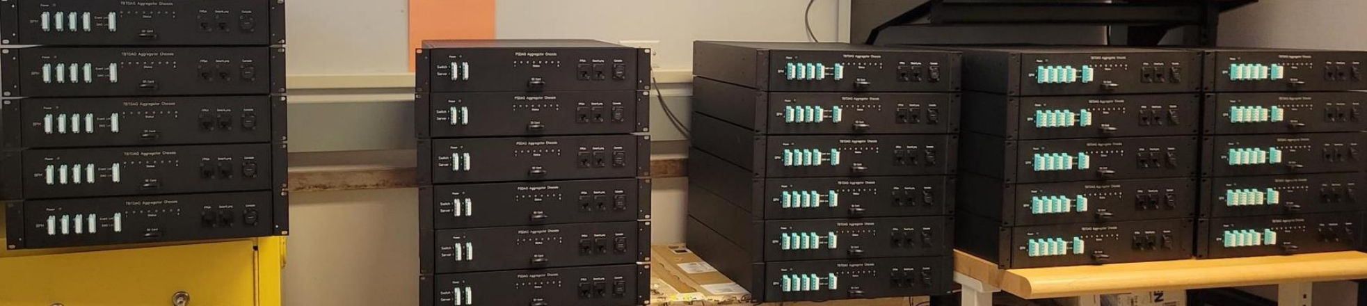
Fully assembled DAQ aggregator FPGA chassis
