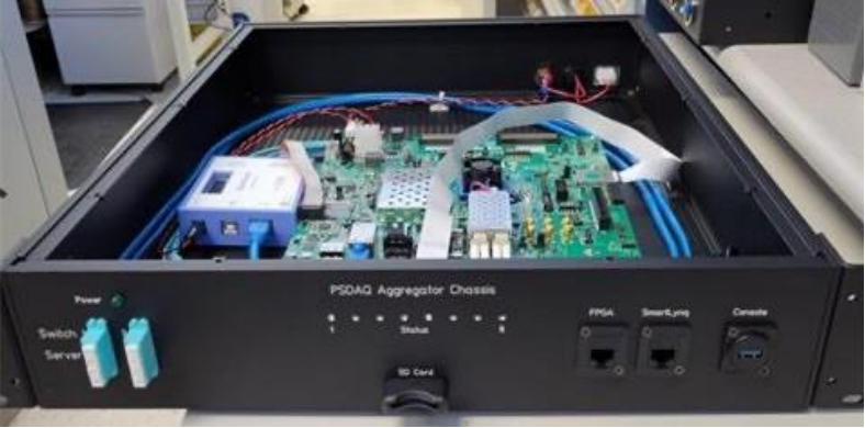
PS DAQ aggregator FPGA chassis
