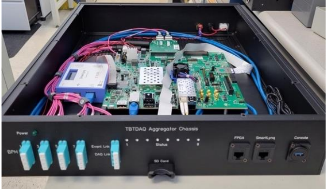
TBT DAQ aggregator FPGA chassis
