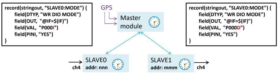
The TTL level signal can be transferred to the other channel or the other node.
