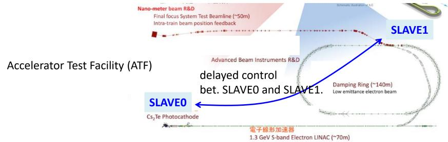
SLAVEO controls before damping ring while SLAVE1 controls after that.
