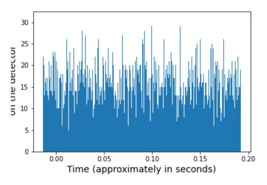
Histograms of time stamps showing statistics of when photons arrive at detector pixels for data in Fig.1. (a) 15 bunch mode with a ring current of 63 mA. (b) Continuous filling mode with a ring current of 68 mA. Courtesy: Chen, Xiaoqian
