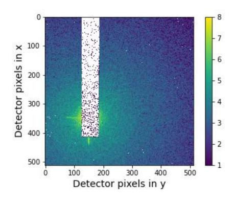
X-ray diffraction pattern from a static ceramic sample on the Timepix single photon counting detector. Data was taken with 15 bunch mode with a ring current of 63 mA. Total exposure time = 3 seconds and the image is in log scale.
