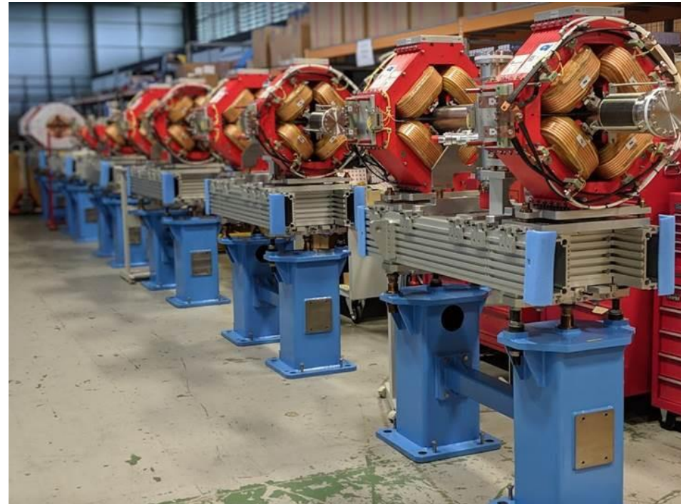
Pre-assemblies of “linac warm units” with magnets.
