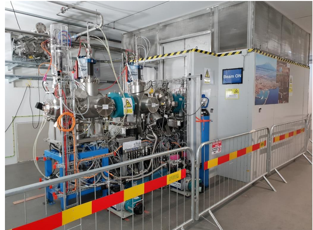
Ion Source & Low Energy Beam Transport (ESS, INFN Catania and CEA Paris collaboration)
