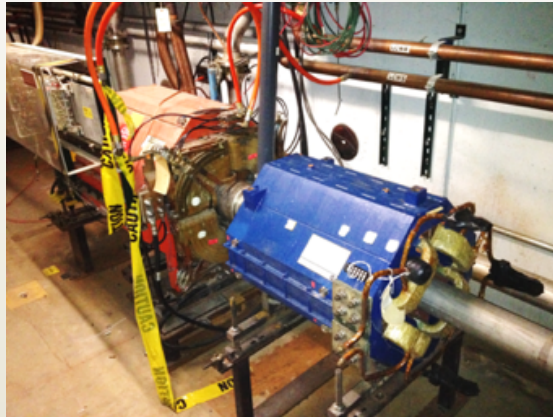
Quadrupole in Delivery Ring used for resonant extraction
