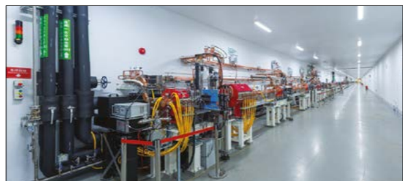
Fig. 3. The SwissFEL C-band linac at the Paul Scherrer Institute (left) and the injection linac for the SINAP XFEL test facility at the Shanghai Institute of Applied Physics (right). Both projects work closely with CLIC to advance high-gradient RF technology.
