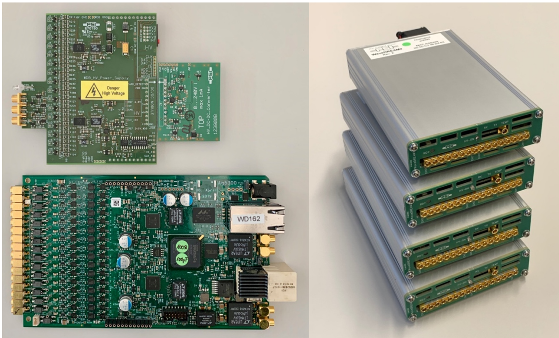
Figure 5: [Left side]: WaveDREAM board (bottom) with 240V high voltage Cockcroft-Walton Generator piggy-back (top). [Right side]: Boxed WaveDREAM boards
