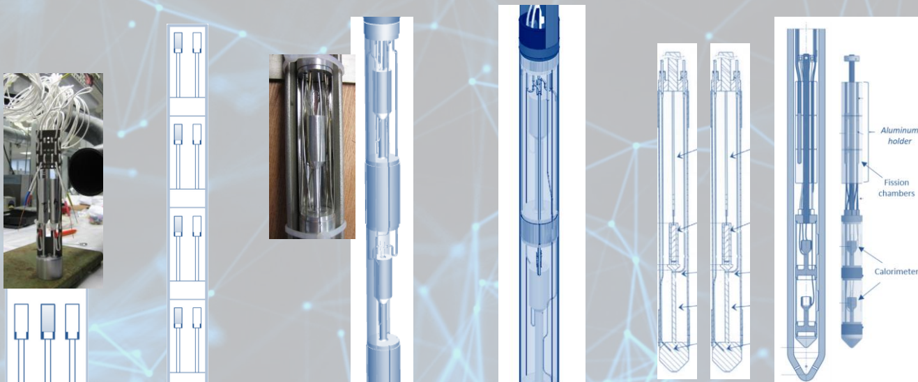
CALMOS 2 calorimeter Sample: Graphite, W, Eurofer, Al, Stainless steel
