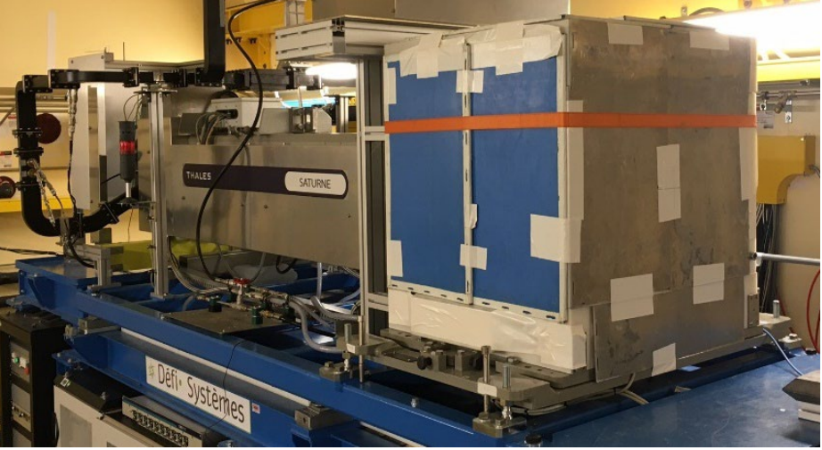
15-20 MeV LINAC with its shielded head
