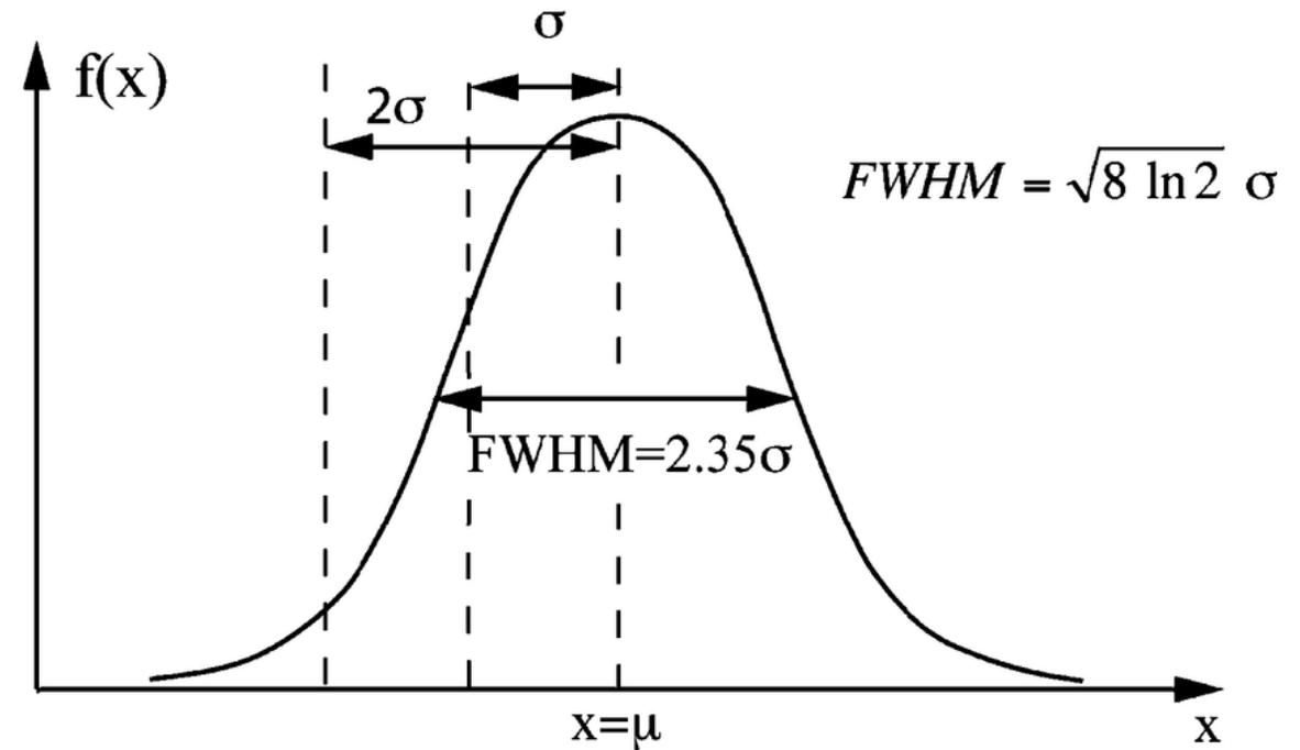
**FWHM** → width of the peak at half of its maximum height in a distribution. FWHM indicates the spread or uncertainty in measurements.
