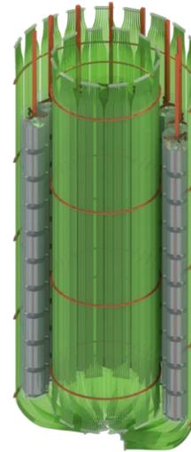
Outer & inner WLS fiber barrel
