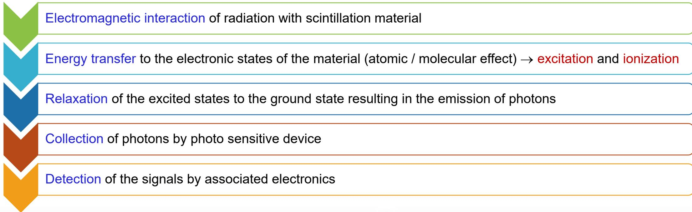
**Scintillation detector:** consists of scintillating material wrapped in a reflective layer, coupled to a light guide, and to a photodetector
