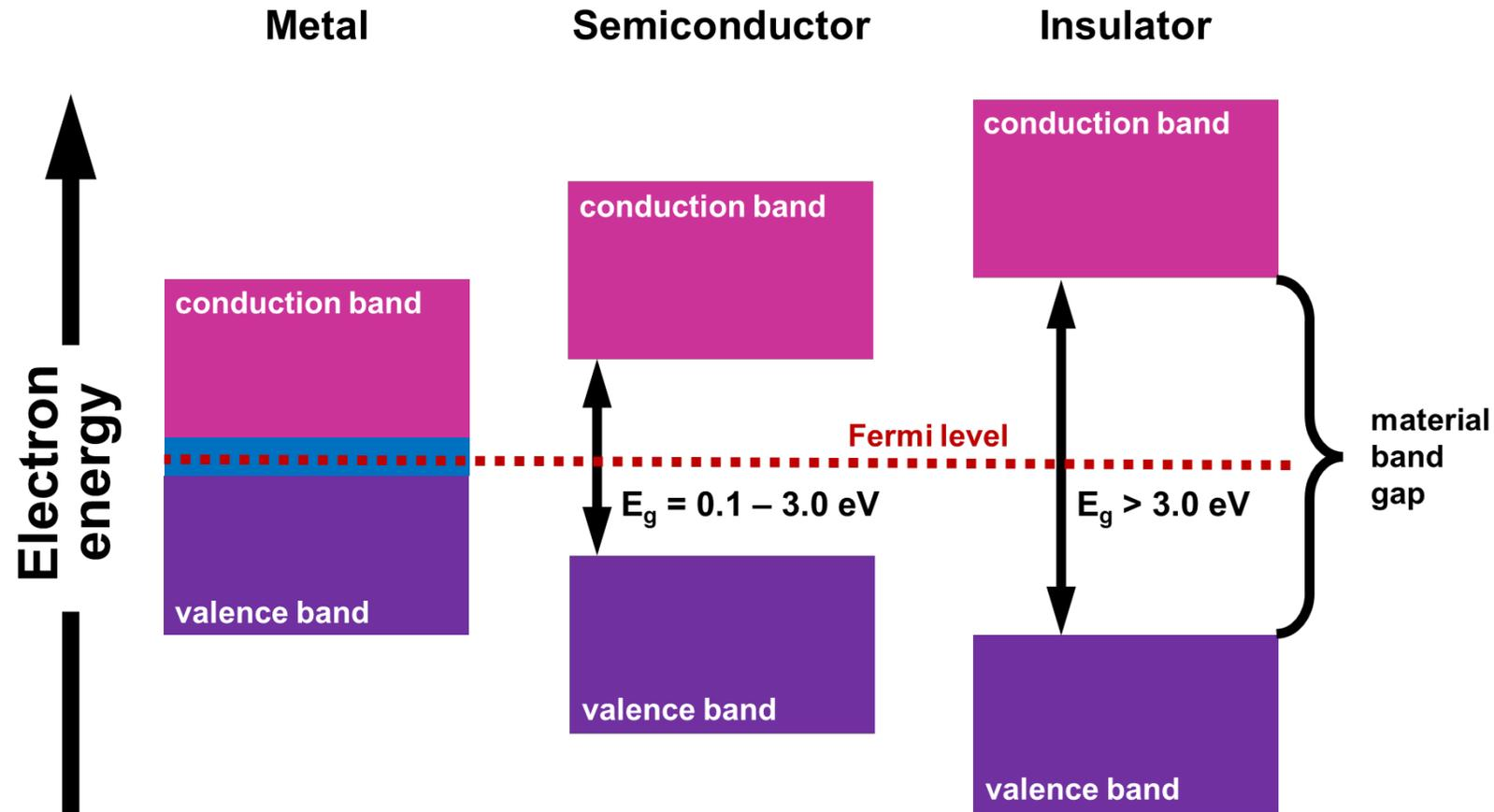
The **Fermi level** is a concept in quantum mechanics and solid-state physics that represents the highest energy level occupied by electrons in a material at absolute zero temperature.
