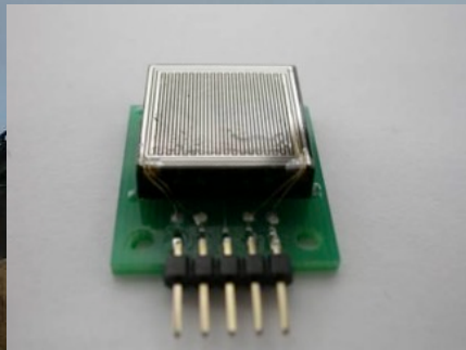
1cm 3 coplanar grid (Cd,Zn)Te detector
