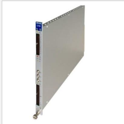
CFB CAMAC-to-FERA Bridge
