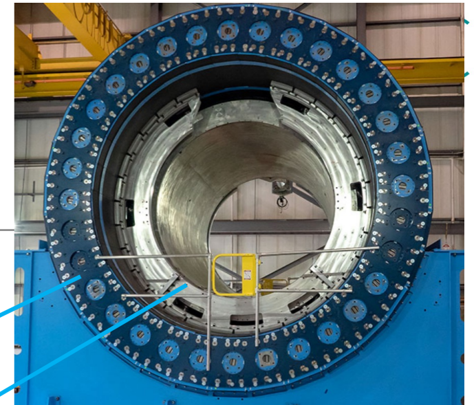
The current sPHENIX carriage with the outer HCal and the magnet
