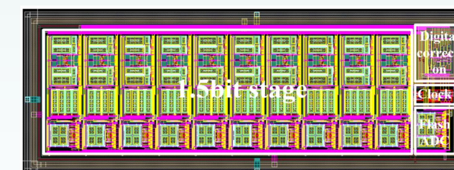
Fig. 6 Layout of the pipeline ADC
