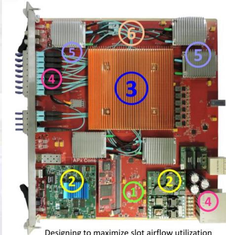
Designing to maximize slot airflow utilization
