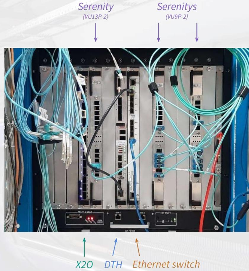
Fig: L1 trigger crate installed at CERN that houses three Serenity, X20, and DTH (DAQ and TCDS hub) board (for multi-board testing)
