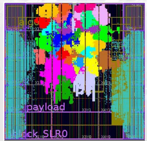
Fig: 39 algorithm placed in 1 SLR (total 117 algorithms for 3 SLR)
