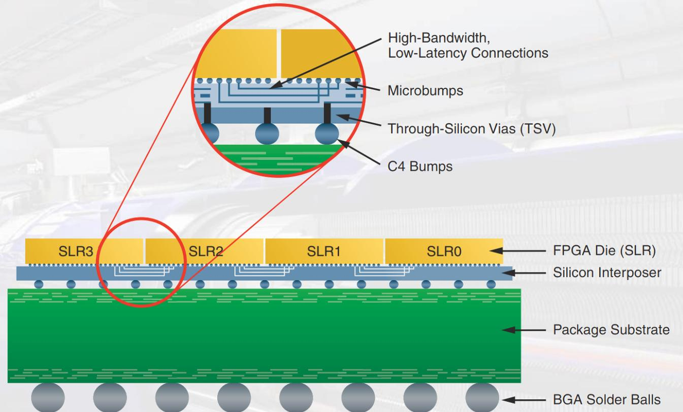
Fig 3: Xilinx FPGA Enabled by SSI Technology\*
