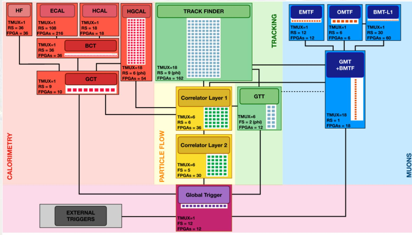
Fig: CMS Phase-2 L1 trigger design. Mentioning the time-multiplexing (TMUX) period, regional (RS) and functional segmentation (FS), and the number of FPGAs for each architecture component.
