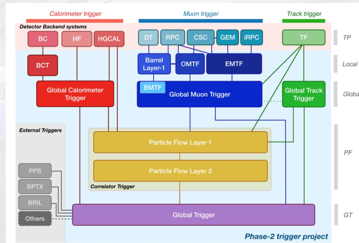
Fig: HL-LHC L1 trigger architecture
