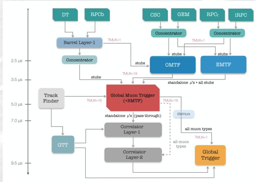
Fig: Muon trigger architecture
