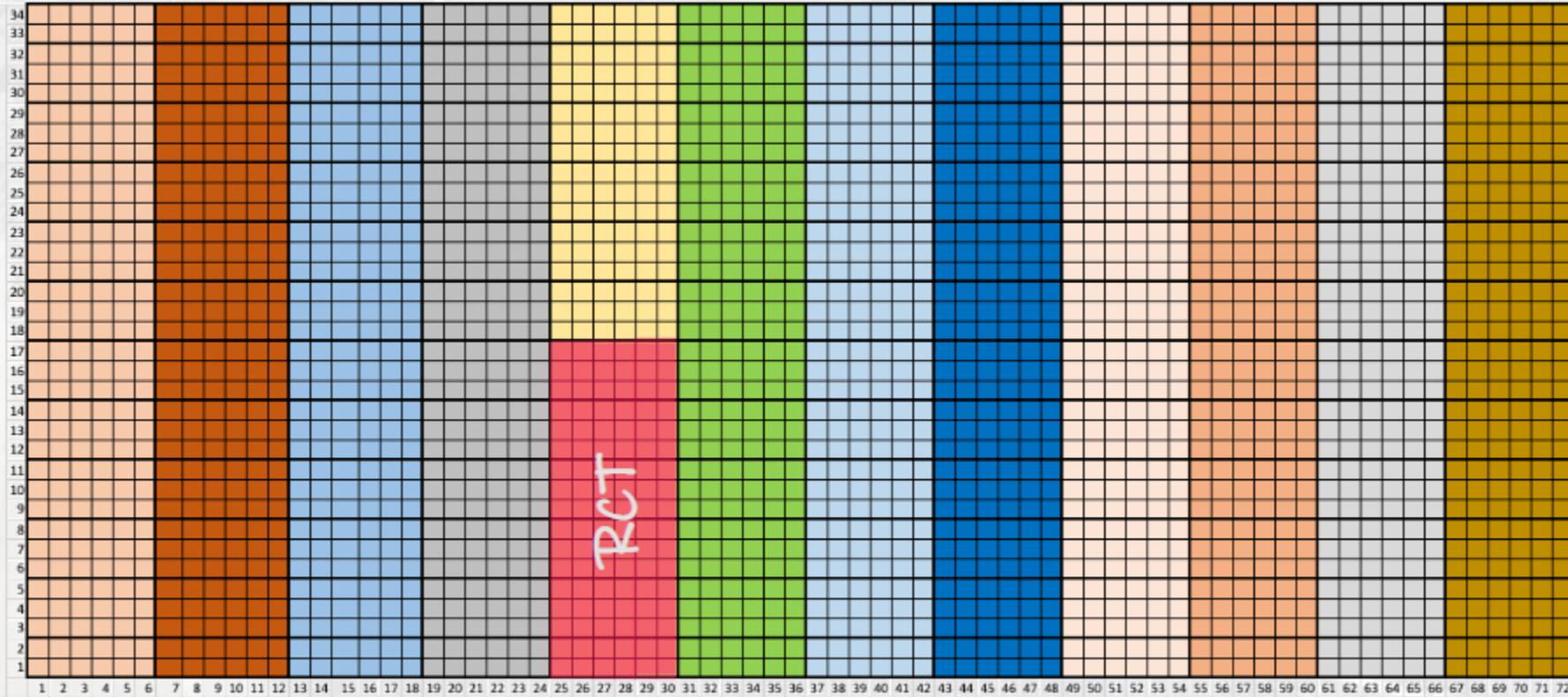
Fig 2: Barrel calorimeter segmentation (new)
