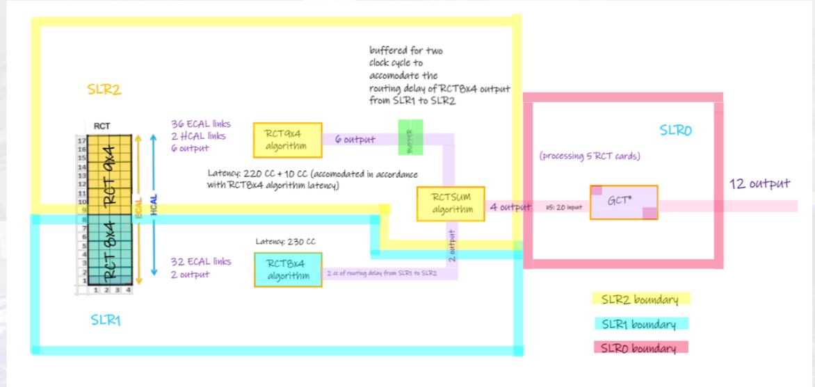
Fig: RCTDR and GCT algorithm implementation in three SLR
