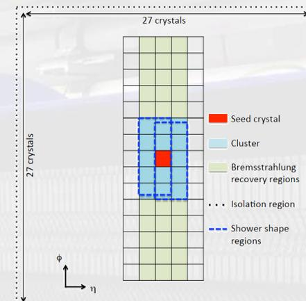
Fig: e/gamma cluster making in RCT algorithm
