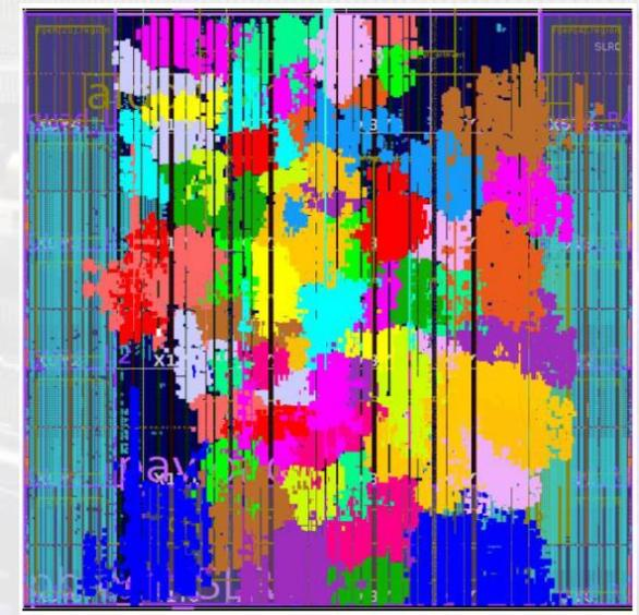
Fig: 78 algorithm placed in 1 SLR (total 238 algorithms for 3 SLR)
