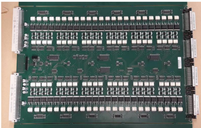
48-channels HV remote board
