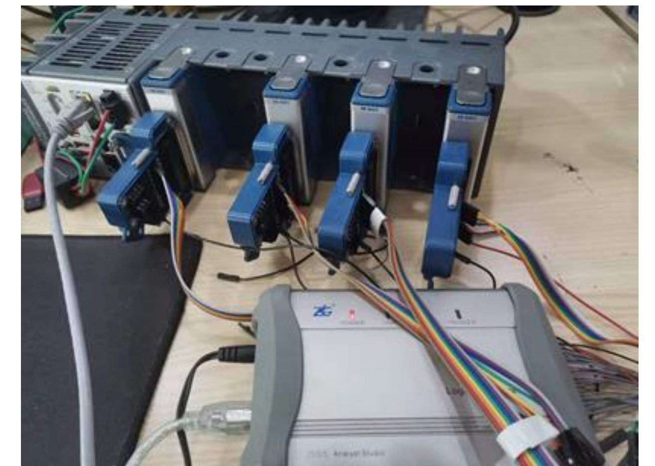
Test of the steady-state operation control system that was based on CRIO.
