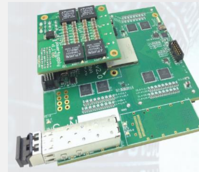
64-channel ADC board
