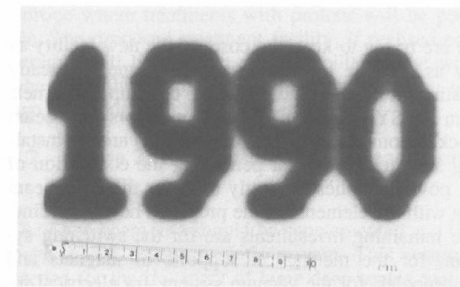
Fig. 4: X ray film irradiated with the 200 MeV proton beam using the spot scanning method.
