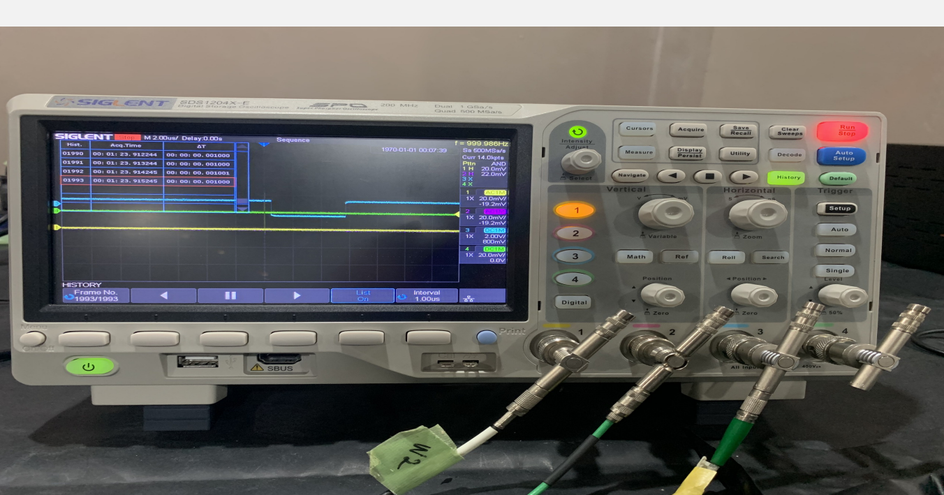
(b) Siglent oscilloscope SDS1104X-E work at both normal (real-time) and sequence modes
