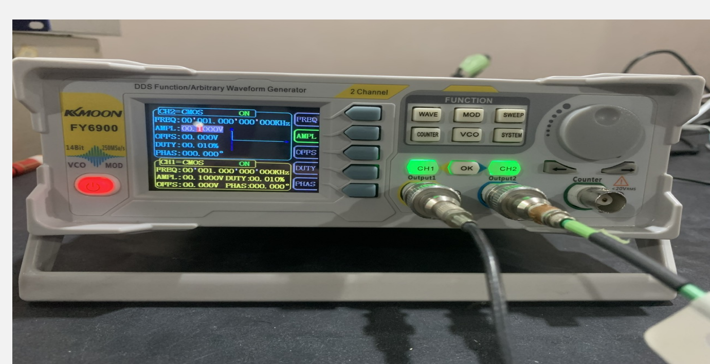
(a) Function generator to generate pulsed signal, mimicking output from photodetectors, with varied frequencies
