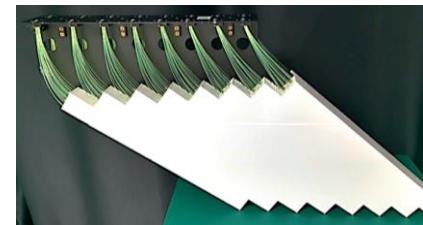
1/6 of the half-sector of the ECal (Zone 8) and single tower structure (Cited from: Y. Li et al 2022 JINST 17 T04005)
