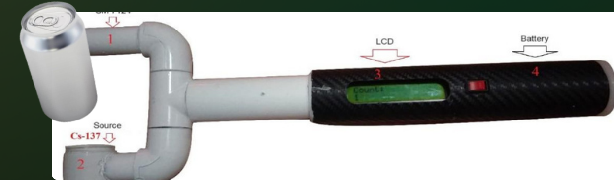
Figure 5. The experimental setup for investigating the handheld level measurement device utilizing the GM7124 counting tube was arranged.
