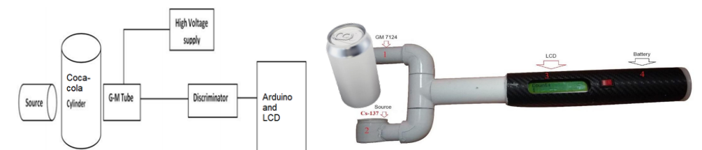
Figure 5. The experimental setup for investigating the handheld level measurement device utilizing the GM7124 counting tube was arranged.
