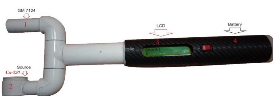
Figure 4. Handheld Liquid Level Measurement Device; (1) GM 7124 counting tube; (2) Cs-137 radiation source 10\mu\text{Ci} ; (3) Count display screen; (4) 9VDC battery pack
