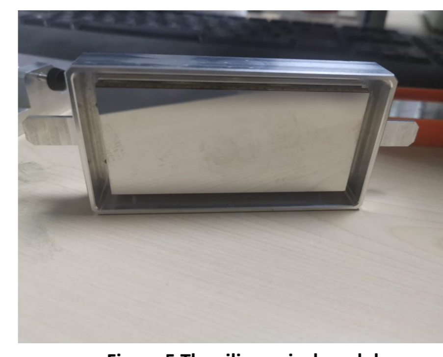
Figure 5 The silicon pixel module
