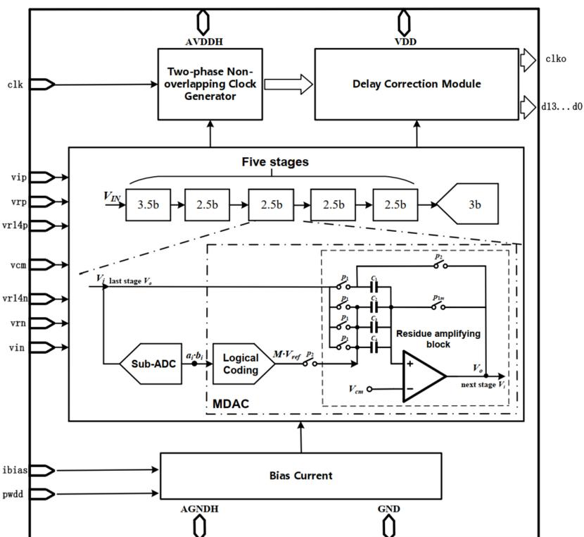
Figure 1. Structure of the pipeline ADC
