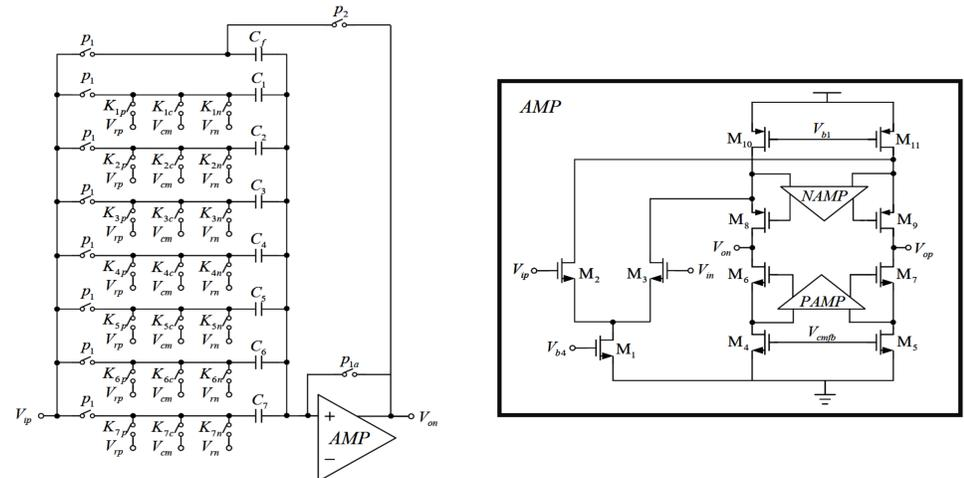
Figure 3. Structure of the first-stage MDAC circuit on one side
