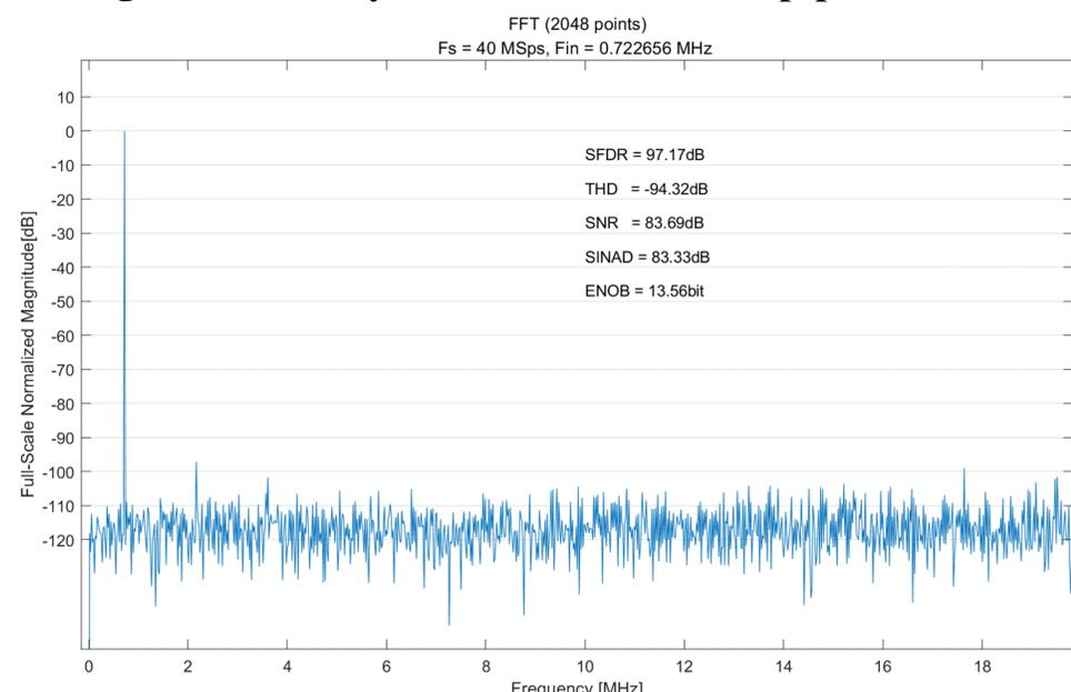
Figure 5. The power spectrum of this ADC
