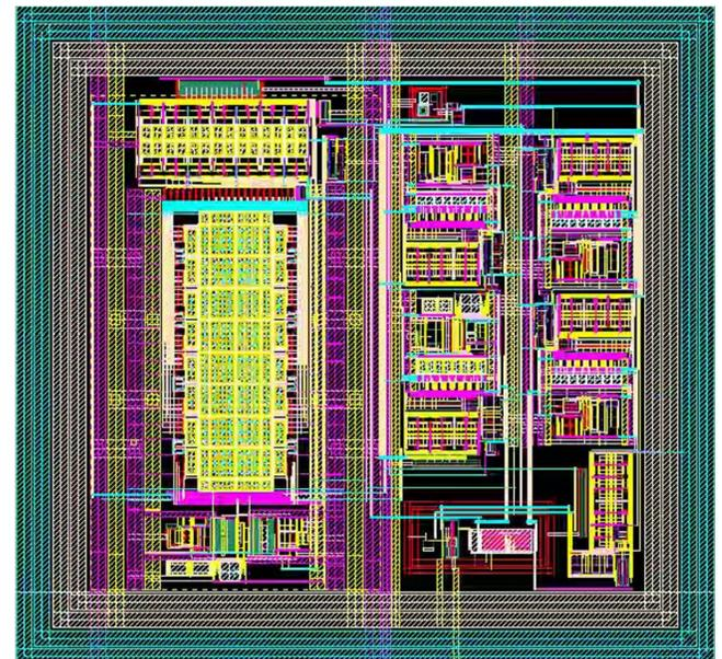
Figure 4. The layout of the core of the pipeline ADC
