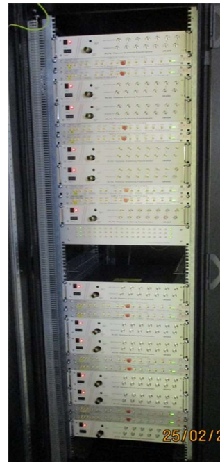
Fig. 17. The integration of 36 Nectarine boards and Polychromators in three thermoregulated cubicles for WEST's C10 experimental campaign is work in progress. .
