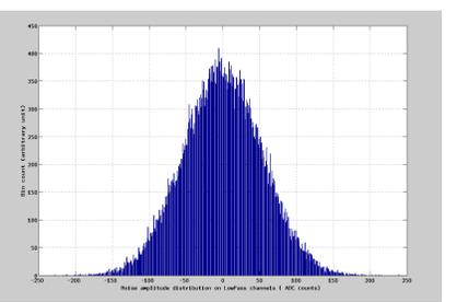
Fig 10 Low pass noise 53.6 ADC counts eq = 34.7uV
