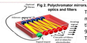
Fig 2. Polychromator mirrors, optics and filters
