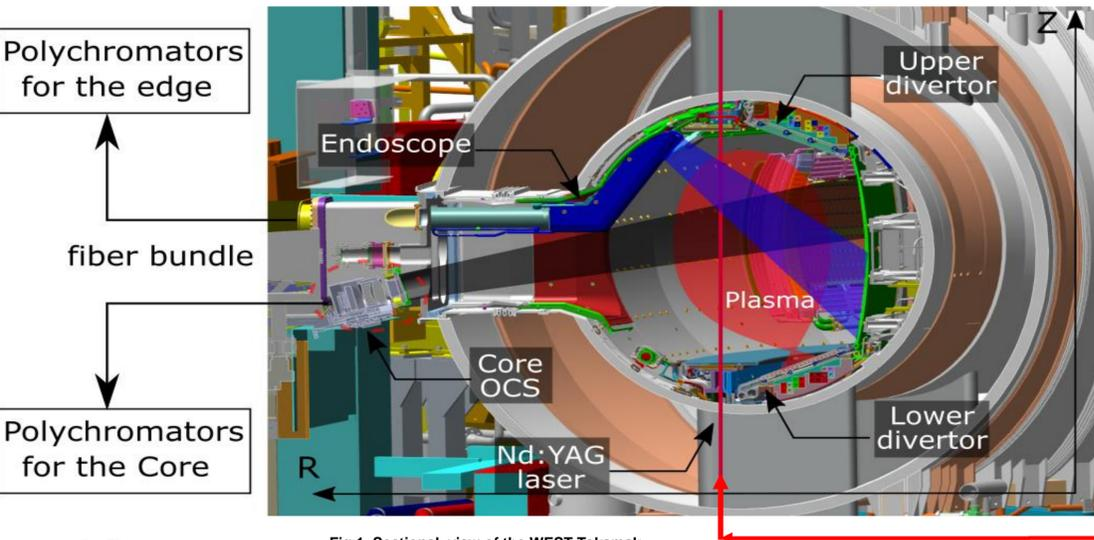
Fig 1. Sectional view of the WEST Tokamak
