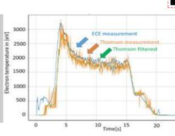
Fig 17. Measurement on plasma Electron Temperature Te (eV) / fct Time (s) for shot 5902
