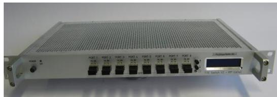
Fig. 6. Front view of a 19" TTE network switch V2 device.
