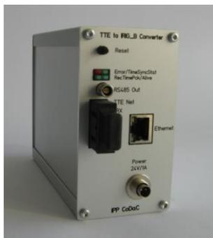
Fig. 9. IRIG-B converter device.
