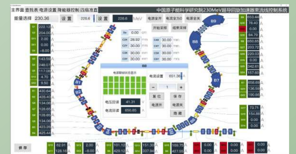
Fig. 7. Control system operator interface
