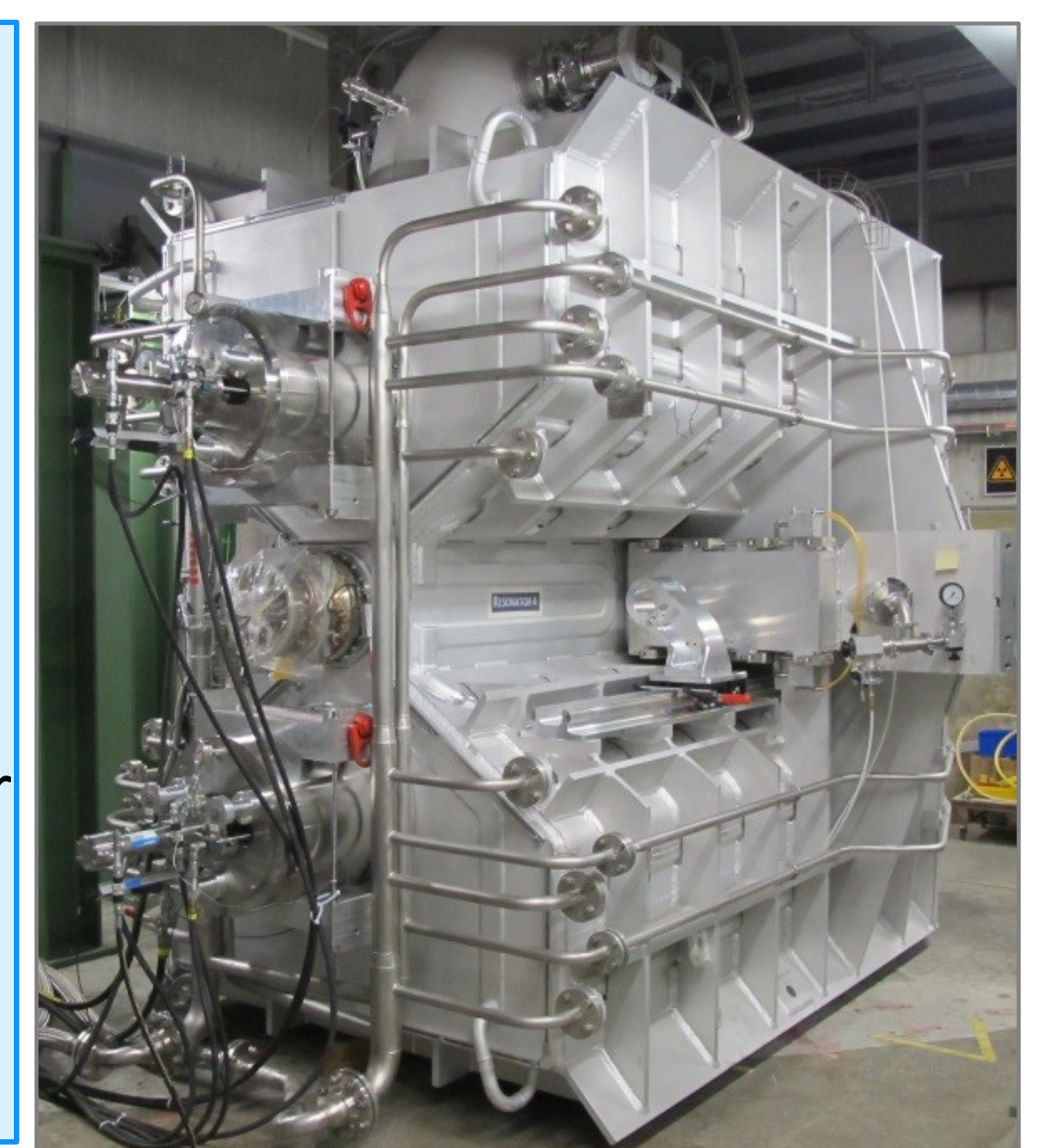
Figure 2: As part of the HIPA upgrade the installed 150MHz 3 rd harmonic cavity will be replaced with a 50 MHz cavity. In further steps all the remaining three cavities of injector 2 will be replaced. The picture shows the 50 MHz accelerating cavity with hydraulic tuners. The whole cavity was built entirely from aluminum. Ideally copper is used due to better conductivity. But the cost of producing such cavities is much higher.
