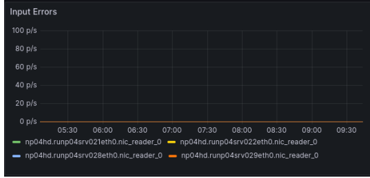
Figure 6: A few hours of a data taking run without errors, consisting 4 APAs of the ProtoDUNE detector at CERN read out by 4 readout unit. The shown metric is an aggregated counter of different error conditions, which also contains the number of dropped and missed packets that may occur due to packet processing performance issues.
