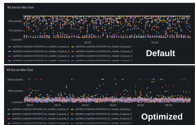
Figure 5: With the optimized NIC hardware and packet processing loop configuration the occurrences of receive bursts resulting with maximum packet counts are drastically reduced. The plots show the number of packets in each burst call from a single interface’s 40 RX queues.
