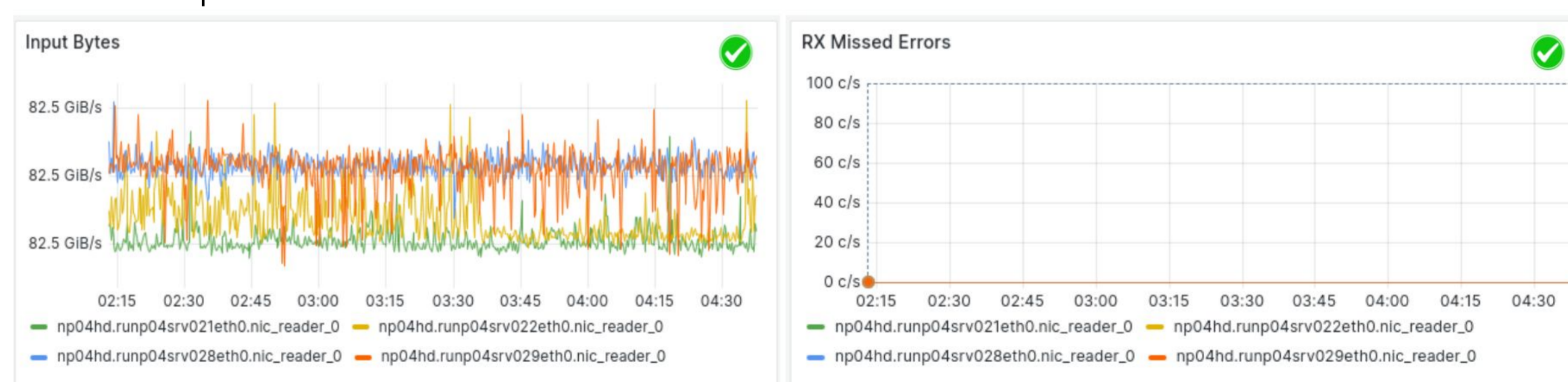
The left plot shows the data rate from 4 detector elements (APAs) of the NP04 prototype detector at CERN. The data is received by 4 readout units, each equipped with a 100Gb NIC. On the right plot the total number of missed packets are shown, which can occur if there is processing backpressure. Both plots indicate that for several hours the full NP04 detector's data was acquired via the Ethernet readout without any data loss.
