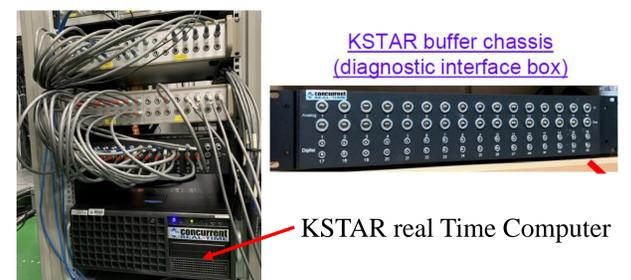
Real-time MHD system on KSTAR computed real-time FFTs from the toroidal magnetics probes for the first time in 2021 for real-time DECAF application.
