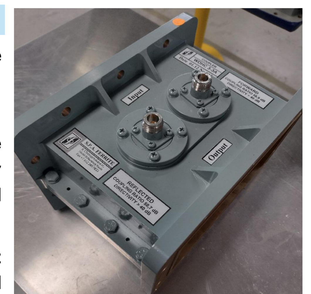
Figure 6) S.P.A. FERRITE, WDC 3-3A bi-directional coupler for 1.3 GHz waveguides used at EuXFEL. The declared directivity is 40 dB. Courtesy of B. Yildirim and V. Katalev
