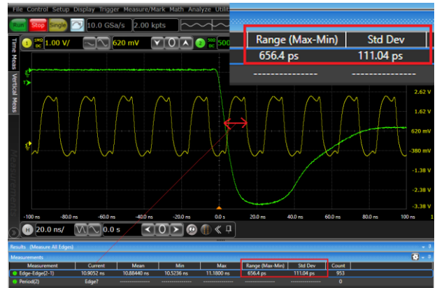
Fig. 3. Clock jitter measurement: Delay of TTCL master trigger (green) against clock on TTCL interface board (yellow).
