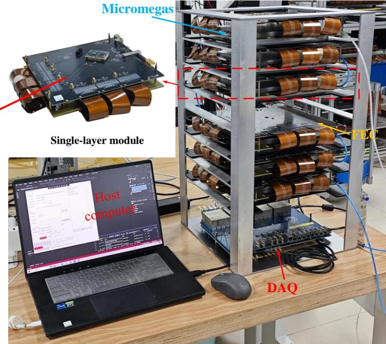
ID: #86 A Compact Readout Electronics based on Current Amplifier for Micromegas Detector
