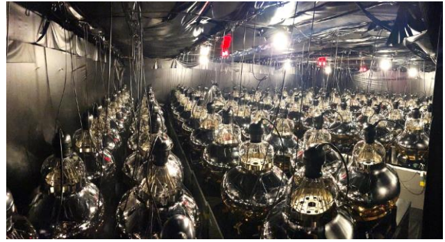
Fig. 5 Facility to check quality of mass production HK PMT. There are 100 PMTs in a room.
