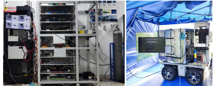
Fig. 4. Left: Muon tomography facility with Micromegas detector, multiplexing circuit, and compact front-end electronics; Right: Muon radiography facility.
