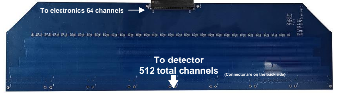
Fig. 3. Encoding circuit multiplexing 1024 detector strips to 64 readout electronics using the complete graph method.
