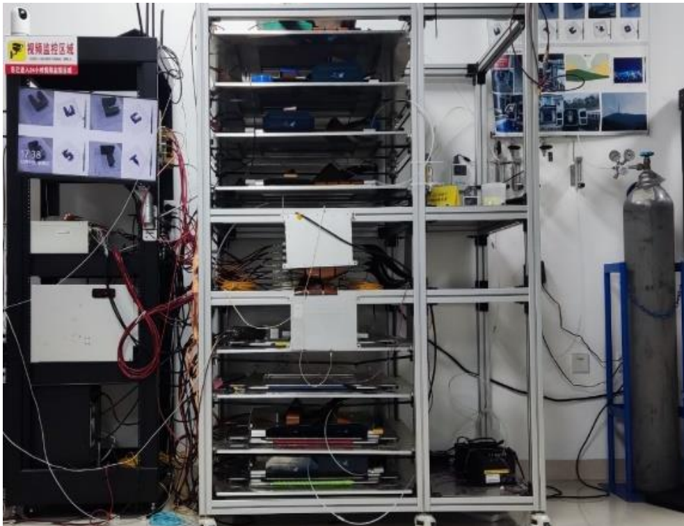
Tomography \mu STC-T-G2 8layer, total number of channel: 16k
