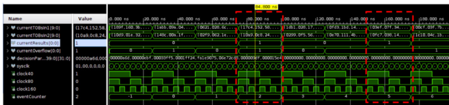
Fig. 21. The simulation waveform of the original decision algorithm, implemented in parallel [17].
