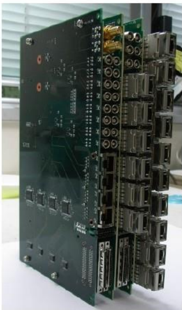
Xilinx Virtex-6 xc6vhx380t, xc6vhx565t 11.2 Gbps with 64B/66B
