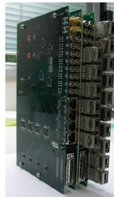
Xilinx Virtex-6 xc6vhx380t, xc6vhx565t 11.2 Gbps with 64B/66B
