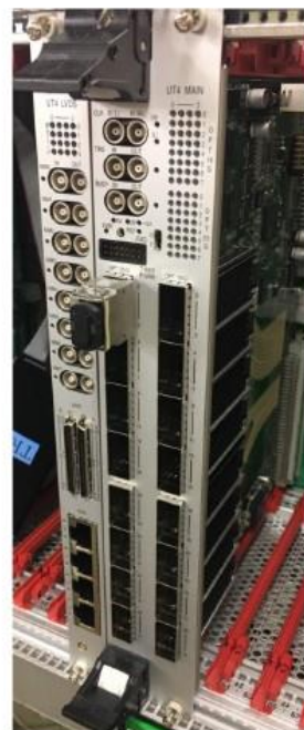
Xilinx UltraScale XCVU080, XCVU160 25 Gbps with 64B/66B
