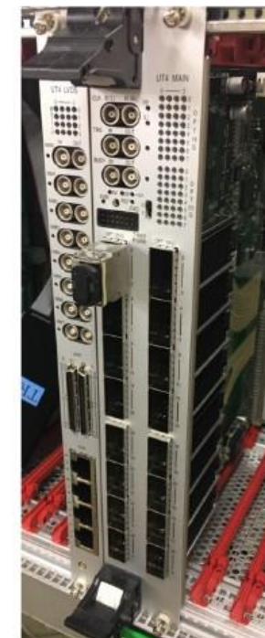
Xilinx UltraScale XCVU080, XCVU160 25 Gbps with 64B/66B
