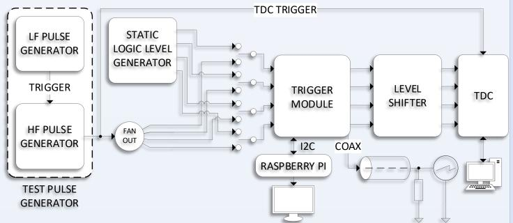
The DTM efficiency is defined as the ratio between the correctly processed events and all events. Burst generator was used during the efficiency test. The number of dynamically generated signals within the individual tracks was changed accordingly to the set logical conditions. The time delay between the DTM input signals was changed in four steps (200/400/600/800 ps) in order to simulate the real CFD signals as they can be slightly shifted in a time domain.
