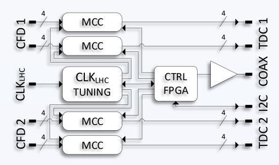
The overall DTM architecture depicted above is based on the multichannel coincidence circuits. These circuits select the events related to the set conditions and subsequently pass/block the train signals on their way to the TDC.
