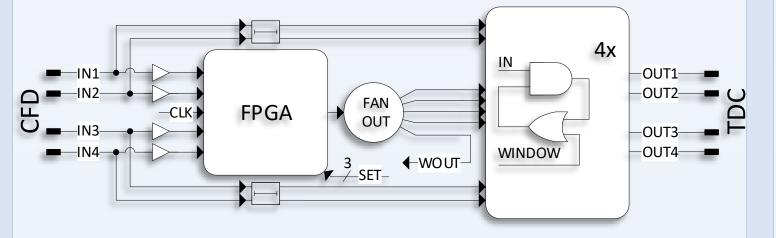
This block diagram illustrates the MCC architecture. The CFD signals are processed in two parallel branches:
