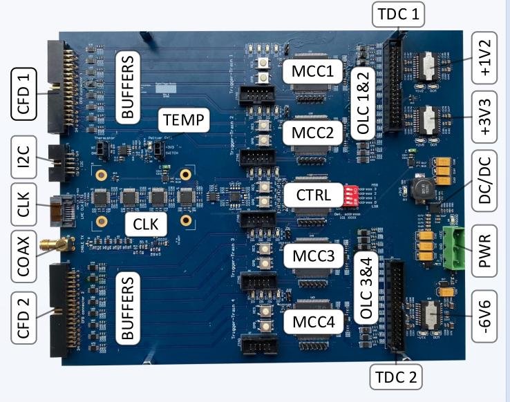
The DTM circuitry is based on the rad-hard (or at least properly tested commercial off-the-shelf) components. The 2-slot NIM box is used as a form factor.
