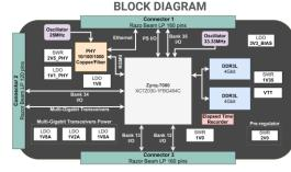
**Onboard Power Supply and Sequencing** Single power supply (5V) operation. Low emissions (EN55022 Class B) shielded switching regulators. Heavy power supply filtering and bypassing. 1.8 V @ 1.5 A and 2.5 V @ 1.5 A supply for external peripherals. Adjustable I/O bank supplies. Fully managed sequencing (including external supplies).
